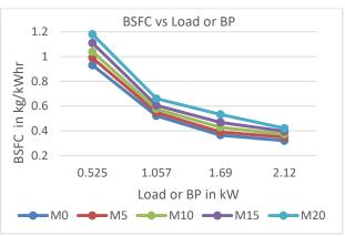
Fig.4 Variation of Brake Specific Fuel consumption with Engine Load
