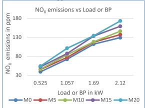
Fig.9 Variation of NOx Emission with Engine Load
