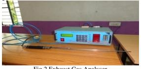
Fig.2 Exhaust Gas Analyser
