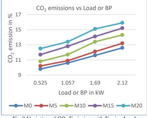
Fig.8 Variation of CO2 Emission with Engine Load
