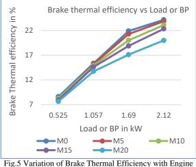
Fig.5 Variation of Brake Thermal Efficiency with Engine Load
